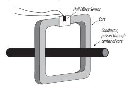
The drawback for Hall Effect technology occurs when the core is subjected to a strong current spike, power surge, or external magnetic field. These forces cause the core's magnetic field to be permanently altered, such that the pre-programmed zero level is no longer accurate. Subsequent outputs from the sensor are skewed. It is possible to recalibrate a damaged sensor, but this involves labor and costly downtime.
