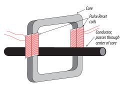
The Pulse Reset coils surround the metal core. As the core's magnetic field fluctuates, the coils periodically demagnetize the core. If a power surge occurs, this frequent neutralization of the magnetic field prevents any lasting effect on the core.
